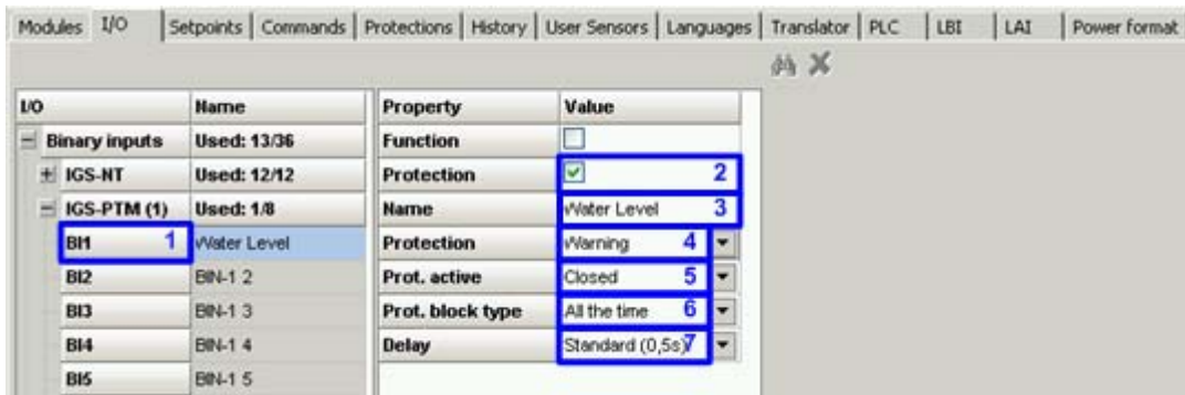
CONFIGURING A BINARY INPUT AS ALARM (PROTECTION)
